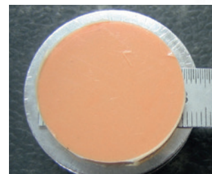
xantasil® shrinkage behavior after several weeks.
